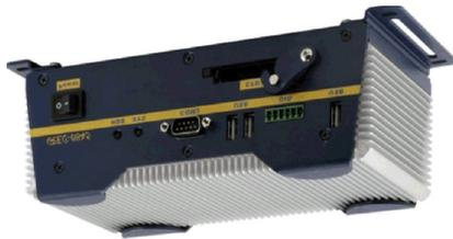
Multifunction gateway with the functions of a data concentrator and protocol converter. Tasks: Combining isolated segments of distributed management systems, data processing in real time with the help of SPS algorithms (according to IEC 61131-3), support through intelligent I / O modules.
